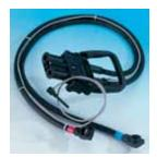
For an optimal charging process of the batteries we recommend the usage of temperature sensors. The temperature is measured at the cell block containers or at the poles for VRLA batteries. For the VLA battery the temperature is measured directly in the electrolyte. It is possible to provide the battery with a completely assembled connection set inclusive a temperature sensor.
